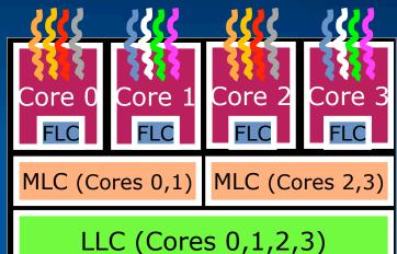
4-threaded, 4-core, CMP Multi-Level Cache Sharing: 4-threads per FLC 8-threads per MLC 16-threads per LLC
