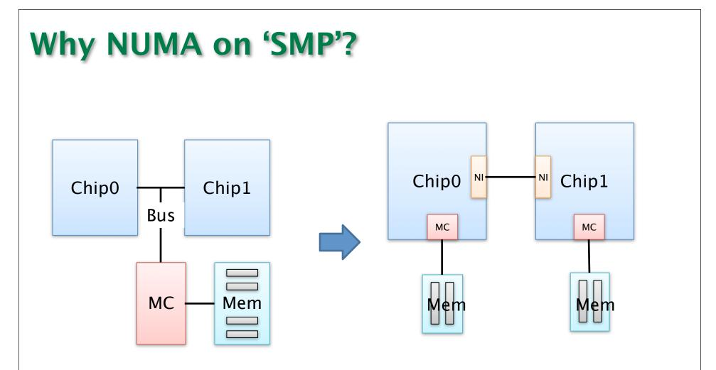
Multi-chip SMP systems used to be bus-based, limiting scalability. On-chip memory controllers improve performance for local data, but non-local data requires communication.
