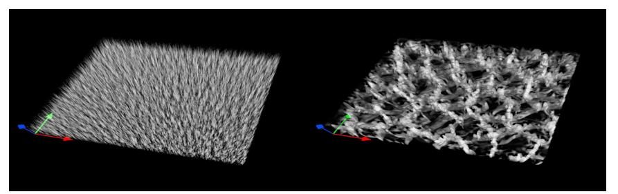
512x512x181 grid visualization – positive vertical velocity over heated plane
