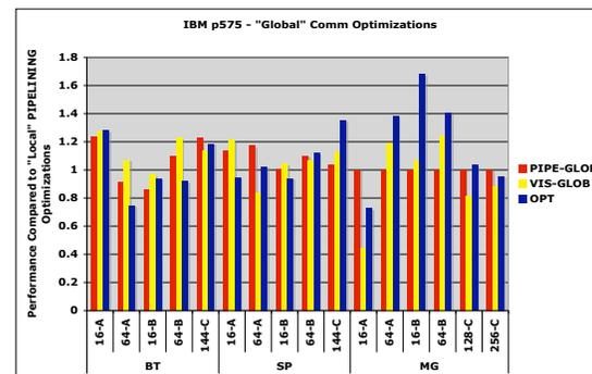
Figure 6: Performance of selected benchmarks using "global" optimization techniques compared to the performance of more "local" optimizations. PIPE-GLOB refers to global communication scheduling using pipelined communication only. VIS-GLOB refers to global scheduling of VIS operations, OPT refers to the performance of compiler generated code.
