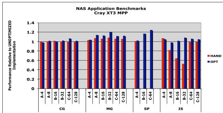
Figure 5: Results for NAS application kernels. Class A on 4 and 8 processors, Class B on 16 and 32 processors and Class C on 64 and 128 processors. Performance (Mops) is reported as relative to that of the officially released version. HANA refers to the best performing manually optimized implementation. OPT refers to the performance of compiler optimized code.
