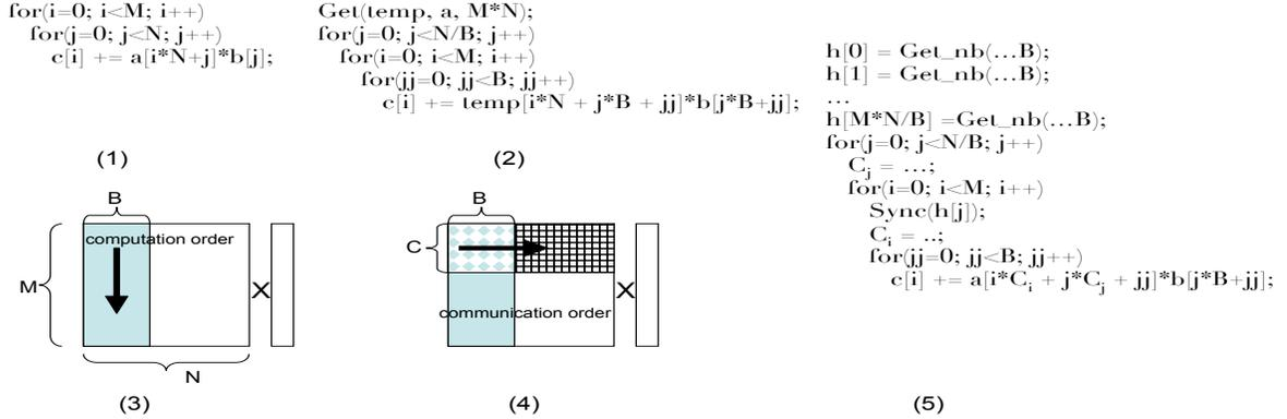
**Figure 2:** (1) Fine-grained loop; (2) Loop after message vectorization and cache blocking; (3) Memory order for cache blocked loop; (4) Possible memory order for packed communication; (5) Code for strip-mined loop;
