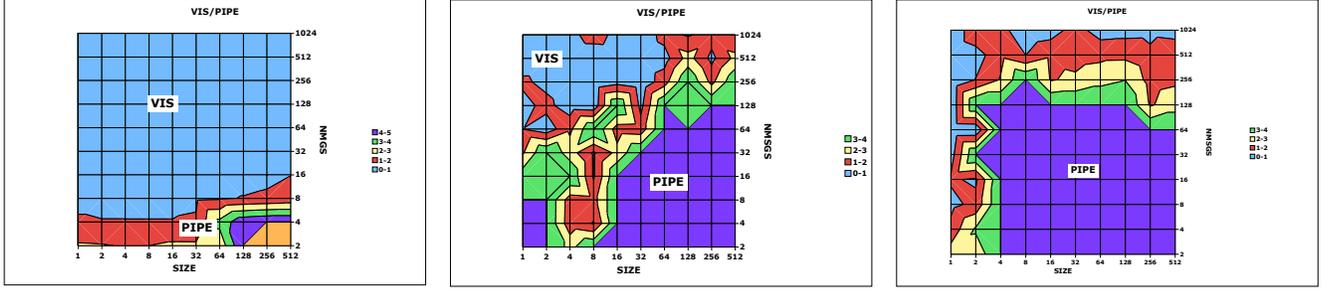
Figure 3: Relative speed of multi-protocol gather on 8 way PowerPC SMP cluster. Color-map represents the ratio  $T_{VIS}/T_{PIPE}$ . Values lower than 1 indicate that the VIS implementation is faster.  $SIZE$  = length of contiguous region in doubles,  $NMSGs$  = number of regions. Left: Inter-node, 1 CPU per node active. Center: Inter-node, 8 CPUs active per-node. Right: Intra-node (SMP only), 8CPUs.
