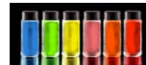
Quantum dots of the same material but different sizes have different band gaps and emit different colors
