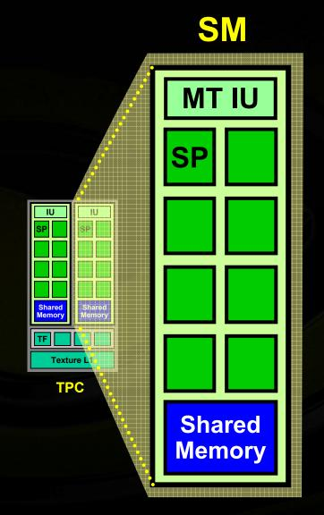
Each SM has 8 Streaming Processors 32 GFLOPS peak at 1.35 GHz **Scalar ISA** load/store architecture **32-bit integer instructions IEEE 754 32-bit floating point** Branch, call, return, predication **Barrier synchronization instruction** 768 Threads, hardware multithreaded 24 SIMD warps of 32 threads Independent MIMD thread execution Hardware thread scheduling **8K registers, distributed among threads 16KB Shared Memory** Concurrent threads share data Very low latency access
