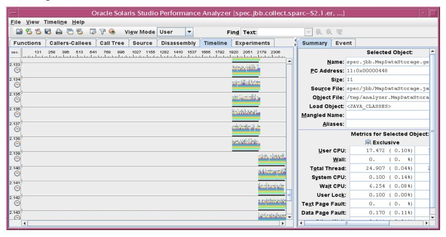
Transition from 15 warehouses to 16 Old threads terminate; new threads are created
